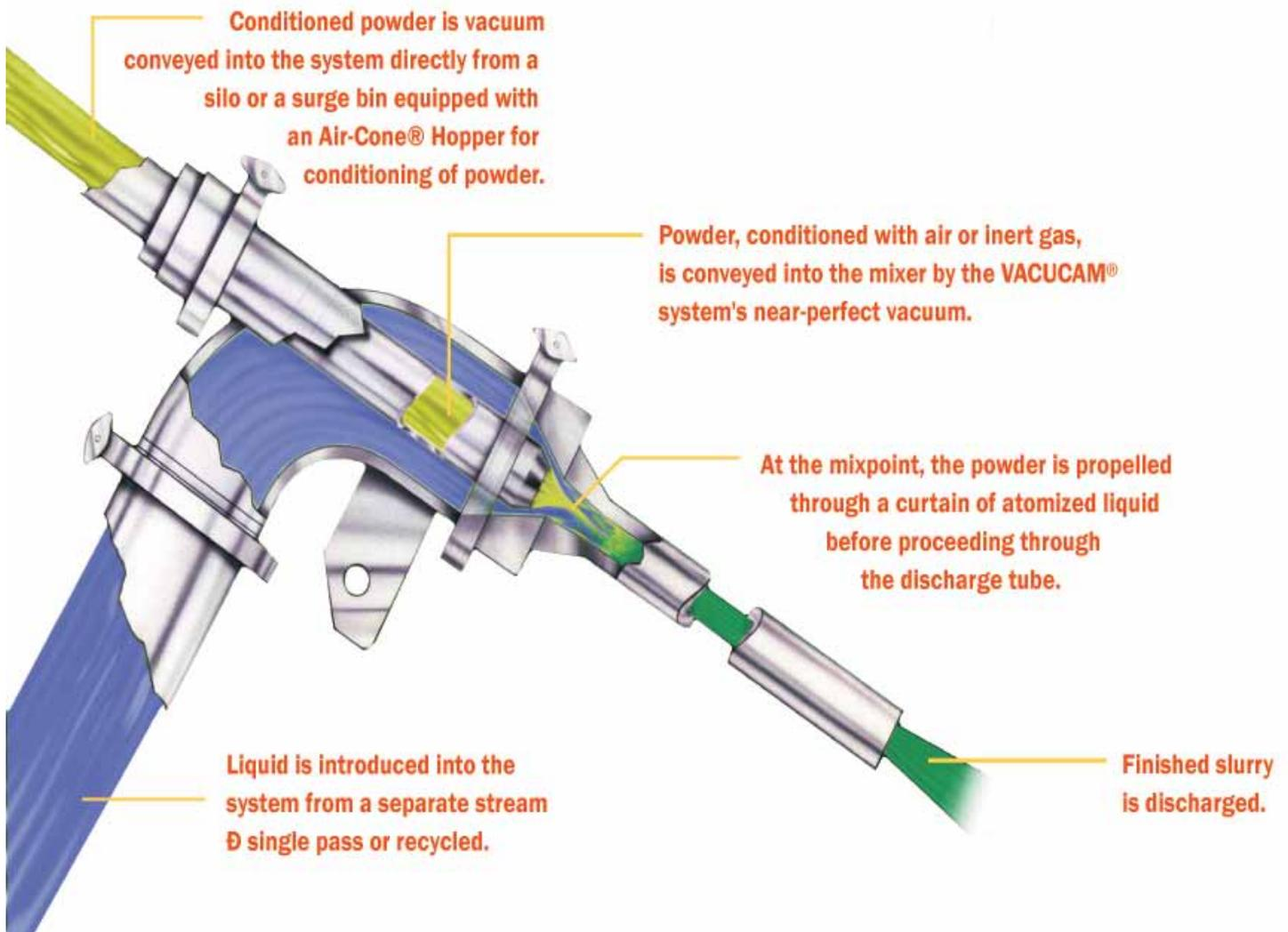
Semi-Bulk Systems can design and integrate the Vacucam® in-line system to feed finished slurry into multiple locations of your preference, such as storage or mix tanks.
