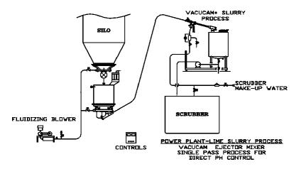
**Mixer Capacities** are available to deliver Limestone Slurries to meet the demand requirements for any size Power Plant. The model 150B/C and the 250C are the preferred choices. The system can be operated with a single mixer or a dual mixer system operating simultaneously. The units are generally selected to operate 12-15 hours/day to meet the 24-hour requirement.
